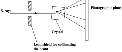
After long exposure to x-rays, the photographic plate is developed and printed. A regular pattern of dark spots called Laue spots are observed around the central dark image. The pattern is due to scattering of x-rays by interaction with electrons in the atom of the crystal. The regularity of the spots implies that atoms in the crystal are arranged in a regular pattern. Consider a beam of monochromatic x-rays incident on a crystal such as KCl at a glancing angle  $\theta$ .
