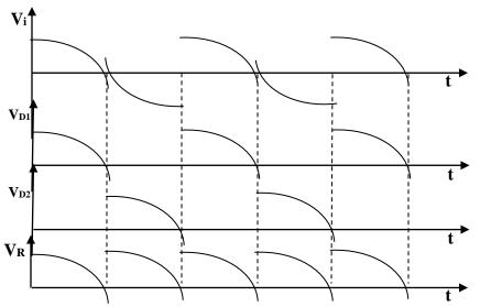
$V_{\text{D1}}$  and  $V_{\text{D2}}$  is output pd due to conduction of diode  $D_1$  and  $D_2$  respectively.
