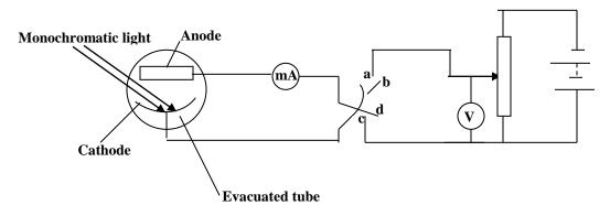
With a connected to b and c to d, the photocurrent I is measured for increasing values of V. A graph of I against V is plotted and has the form shown below;
