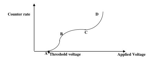
Below a certain value of p.d known as *threshold voltage*, no counts are recorded at all since the number of ions produced per second is not enough to produce sufficient current which can result in a pd of sufficient magnitude to be detected.
