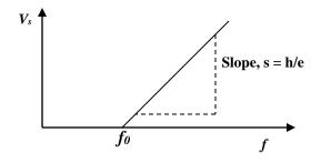
The slope of the graph, s = h/e, where e is the electronic charge Hence Planck's constant, h = se. For different metal surfaces we obtain,
