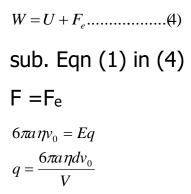
After repeating the experiment for different oil drops, Milkan found out that the charges on the drop were integer multiples of the value  $1.6 \times 10^{-19}$ C. This value was taken to be the basic charge and is the charge on the drop.
