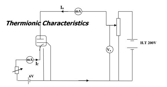
Keeping the filament current If constant, the p.d V<sub>a</sub> between the cathode and the anode is varied. The corresponding anode current I<sub>a</sub> is measured. A graph of I<sub>a</sub> against V<sub>a</sub> constitutes the anode – current anode voltage characteristics. By setting the filament current to other constant values, the corresponding I<sub>a</sub>-V<sub>a</sub> characteristics can be obtained. These features can be shown below
