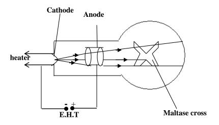
If an opaque object (Maltese cross) is placed in the path of the cathode rays, a sharp shadow of the Maltese cross is cast on the screen.
