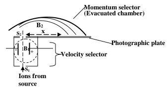
Ions from the source enter the velocity selector through collimating slit s<sub>1</sub>. The ions enter the velocity selector and only ions with velocity  $v = \frac{E}{B_1}$  pass through undeflected. E is the electric field intensity of electric field in the momentum selector, B<sub>1</sub> is the magnetic flux density of the magnetic field in the velocity selector.
