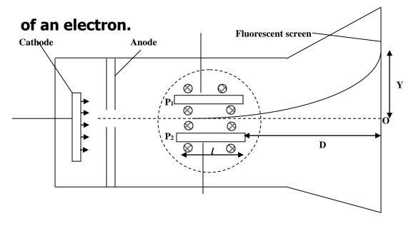
Electron emitted by the heated cathode is accelerated to the anode. In the absence of the electric and magnetic fields, the cathode rays strike the florescent screen at O. The p.d is then applied between plate's  $P_1$  and  $P_2$ . The deflection Y of the cathode rays is measured. A magnetic field is then applied to the plane of the figure by passing current through a pair of circular coil one on each side of the glass tube.
