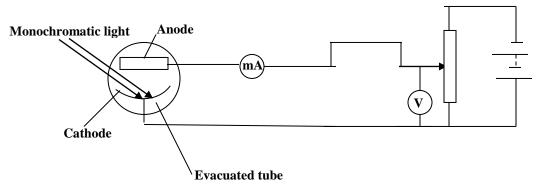
The anode is at a negative potential with respect to the cathode. The pd between the cathode and anode is varied until the photocurrent recorded by the ammeter is zero. The value of Vs of the voltmeter when this occurs is noted. The experiment is repeated for monochromatic light of different frequency, f but same intensity. A graph of Vs against f is plotted
