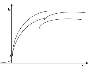
For Va = 0, electrons are emitted by the cathode with a range of speeds. A few of the electrons are emitted with sufficient kinetic energy to be able to reach the anode. This leads to a small current. If the anode is made negative relative to the cathode, a reverse current exists for negative potentials up to about 0.5V and then decreases to zero.
