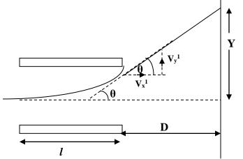
The time taken by the electron to move through the plates  $t_1 = \frac{l}{u_2}$
