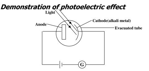
When light falls on a metal cathode, a galvanometer shows a deflection, indicating flow of current. However when the plates are covered, more current flows. Energy of the incident light is absorbed by the electrons and instantly an electron jumps out. Such ejected electrons are called photoelectrons.
