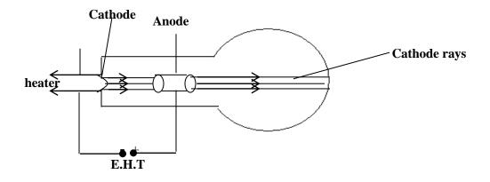
The electrons are produced at the cathode by thermionic emission and are accelerated towards the screen by the anode which is connected to the terminal of the extra high tension battery. The thermionic emission is the process whereby metal surfaces emit electrons when heated.
