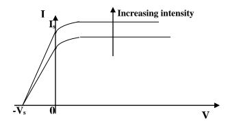
The curves saturate early meaning that a small voltages is sufficient to collect all the electrons emitted. The photocurrent is not zero when the voltage is zero. The photocurrent persists even when the anode is negative relative to the cathode. This is because electrons are emitted with sufficient kinetic energy which overcomes the opposing electric field and reach the anode.
