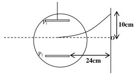
In the figure,  $p_1$  and  $p_2$  are metal plates each of length 2cm and separated by 0.5cm in a uniform magnetic field of flux density 4.7 x  $10^{-3}$ T.
