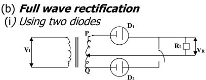
When P is at negative potential relative to Q, diode  $D_1$  conducts whereas  $D_2$  doesn't.
