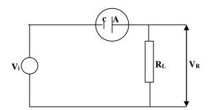
During the half cycles when A is positive relative to C the diode conducts and a p.d V<sub>R</sub> appears across the load R<sub>L</sub>. During the half cycles when A is at a negative potential relative to C, the diode does not conduct and no p.d appears across R<sub>L</sub>. The a.c is half-wave rectified.
